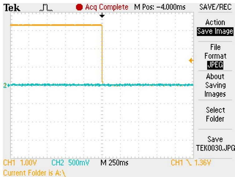
Fig 6: Shutdown Pop Noise absent using PA4201
