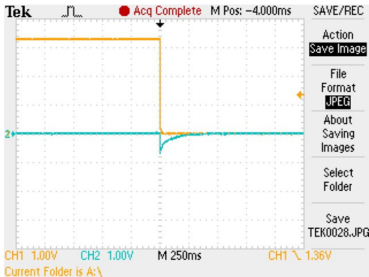
Fig 4: Shutdown Pop Noise observed at Line Out
