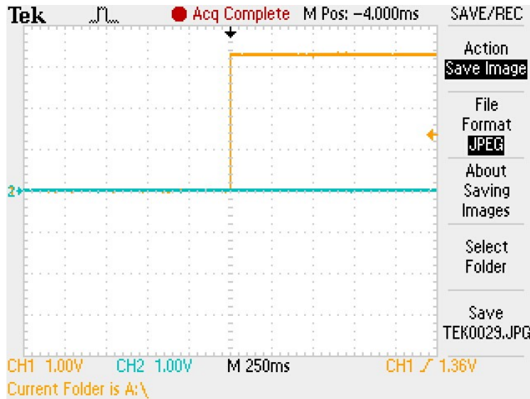
Fig 5: Startup Pop Noise absent using PA4201
